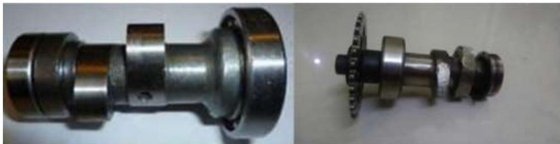
Fig. 3: Actual and Modified cam
