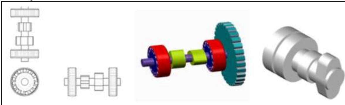
Fig. 2: Model of dual lobe cam
