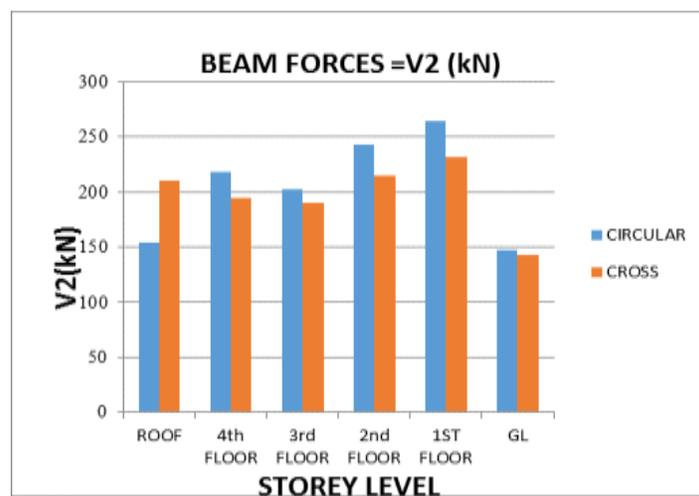
Chart 5: Max. shear force -V2-(kN) in beams
