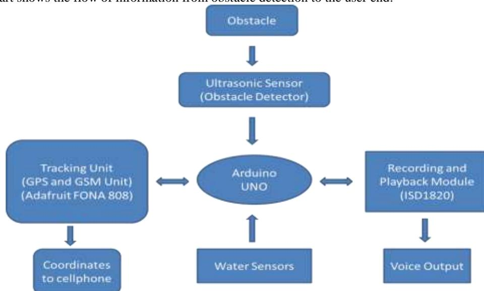
Fig. 3: Information flow from device to the user
