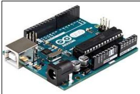
Fig. 4: Arduino UNO board
