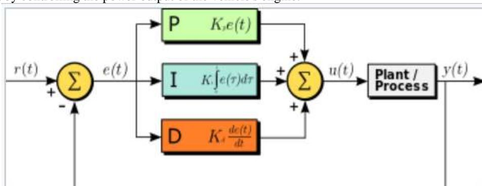
Fig. 1: Block Diagram of a PI Controller
