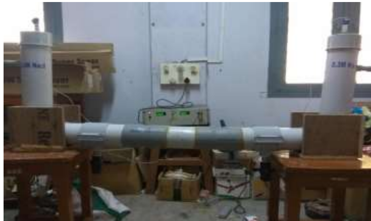
Fig. 4.5: Rapid chloride permeability test setup
