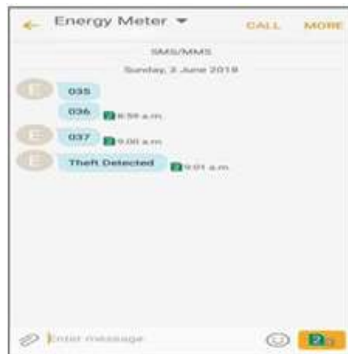
Fig. 7: Power blinking rate and theft detected part displays on consumer mobile as SMS.
