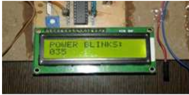
Fig. 5: LCD display of energy meter power blinking rate
