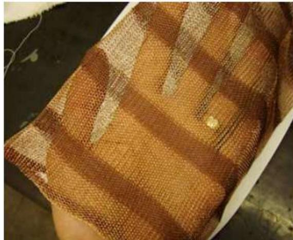
Fig. 3: Example of Vertically Embedded Conductive Bands
