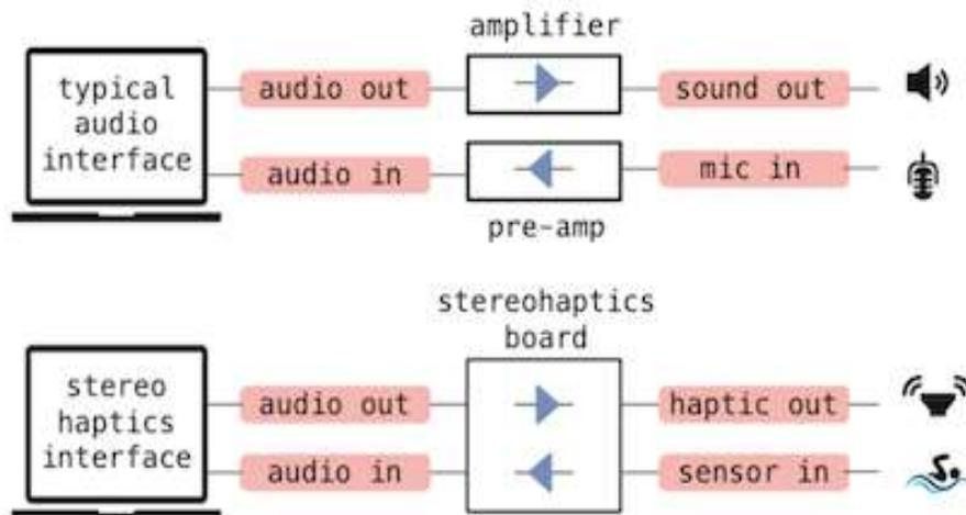
Fig. 2: Haptic Audio Interface
