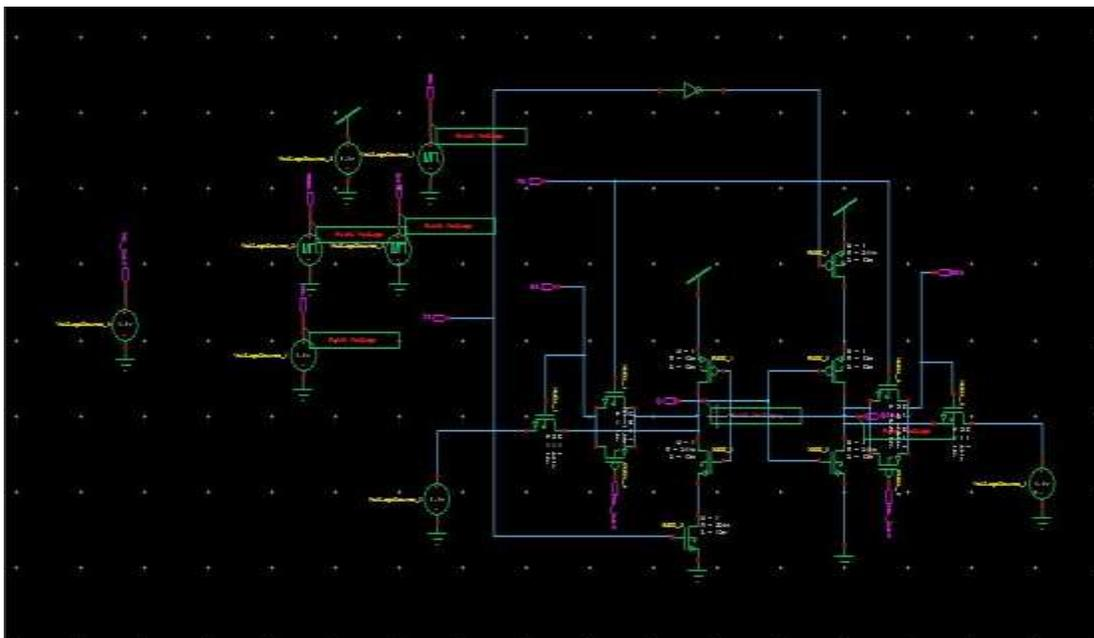
Fig. 3: The proposed 12T SRAM cell.
