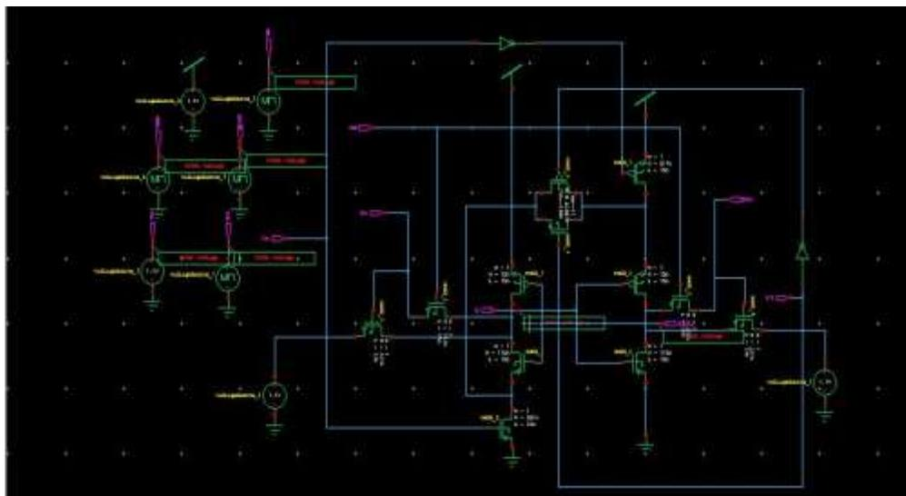
Fig. 1: The 12T SRAM cell.
