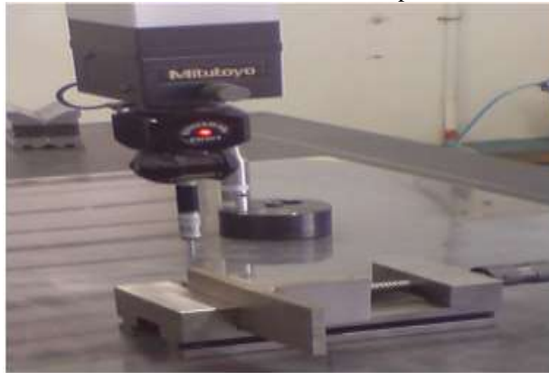
Fig. 3: Contour measurement using CMM
