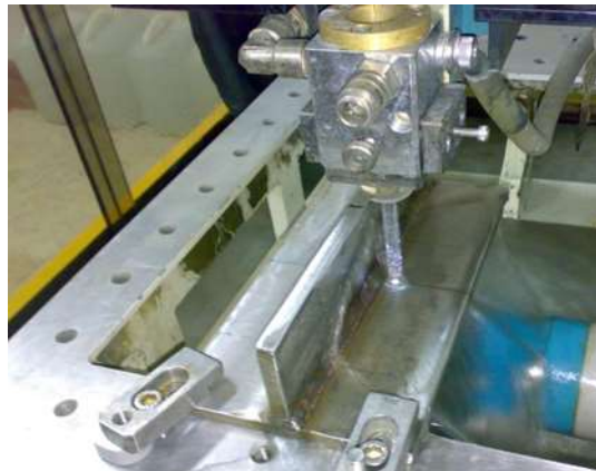
Fig. 2: Wire cut EDM of DSS2205T- Joint
