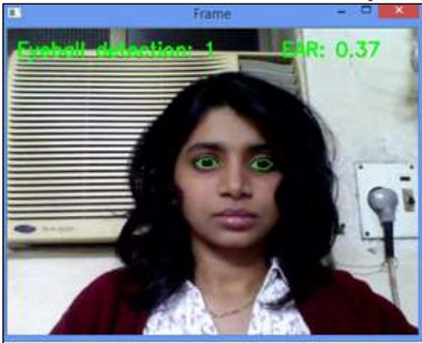
Fig. 2: Eyeball detection  $EAR > 0.2$  (Threshold)
