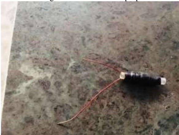
Fig. 3: Hollow cylinder wrapped with wire and ends sticking out
