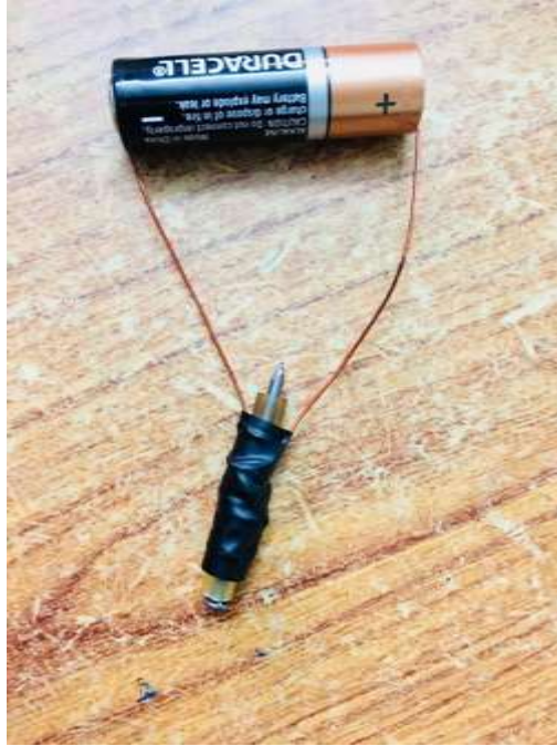
Fig. 5: Closed circuit, showing nail pulled inside as soon as voltage is applied to circuit
