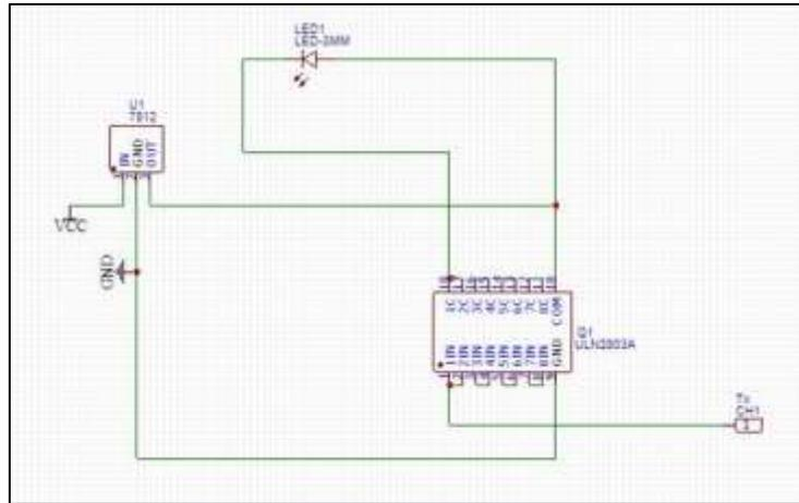
Fig. 3: Transmitter circuit
