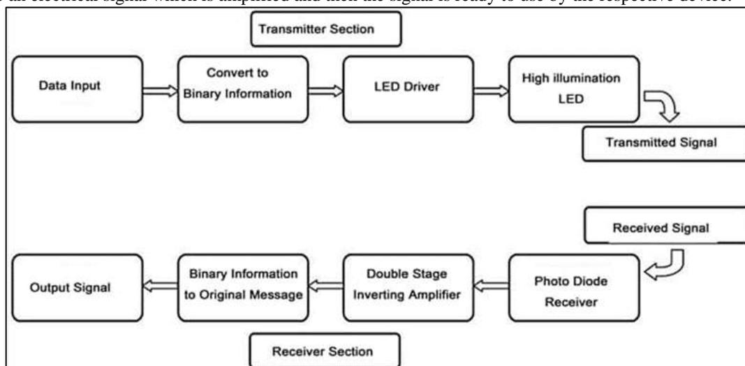
Fig. 2: Block diagram of basic Li-Fi system.
