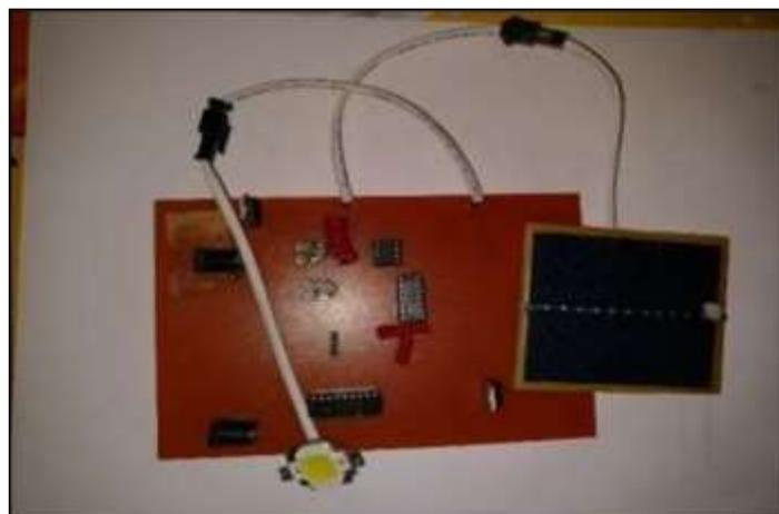
Fig. 5: Hardware model of the transceiver circuit.
