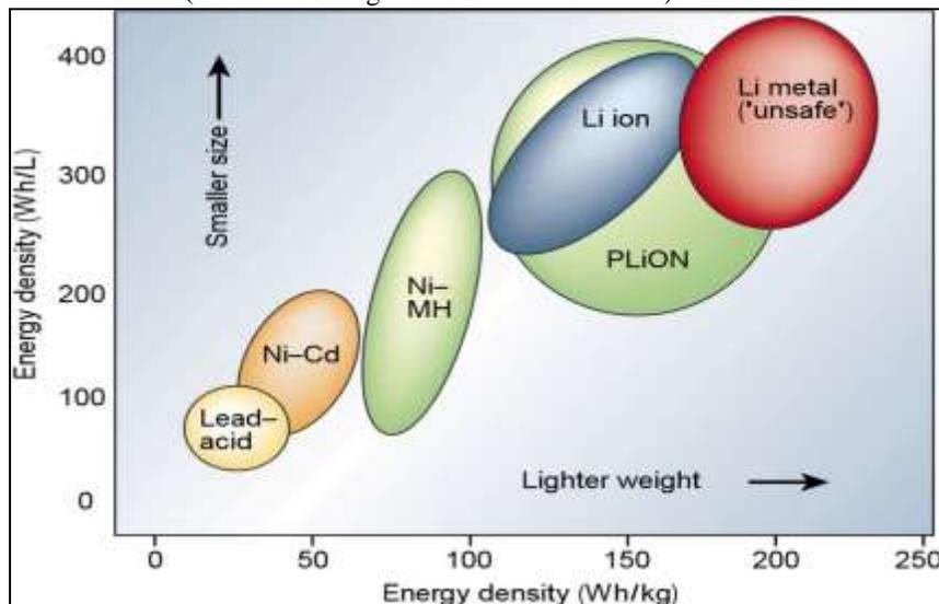
Fig. 1: Energy Diagram of Different Battery Weight & Size
