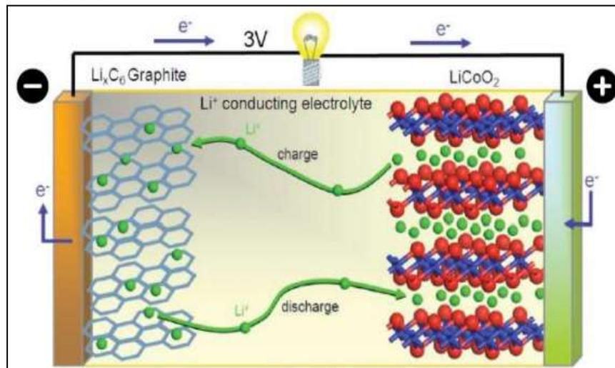
Fig. 2: Schematic of Ions (Charge & Discharge) & Electrons (Discharge) Movements in a Lithium Ion Cell
