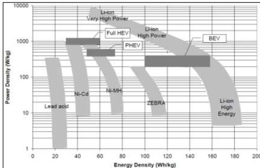
Fig. 3: Power & Energy Densities of Battery Technologies
