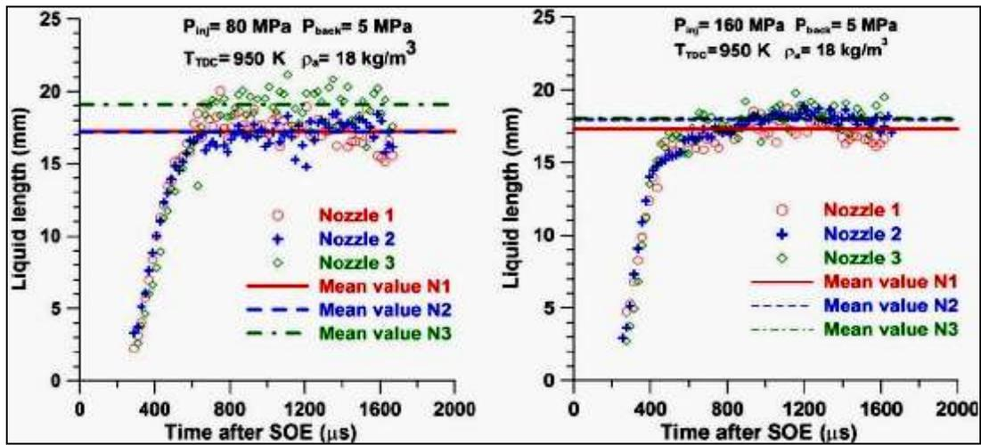
Fig. 4: Examples of Liquid Spray Penetration Results
