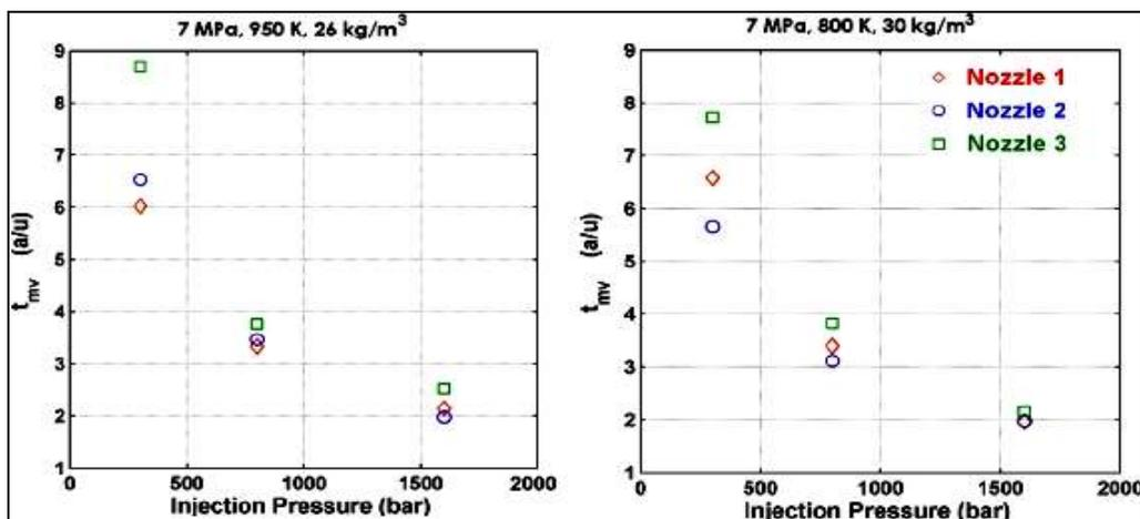
Fig. 5: Time to Mix and Vaporize in Terms of Injection Pressure
