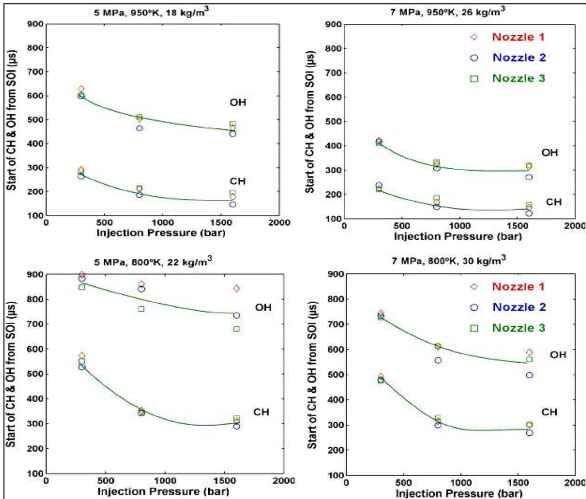
Fig. 6: CH- Appearance (below) and Ignition Delay (Above)
