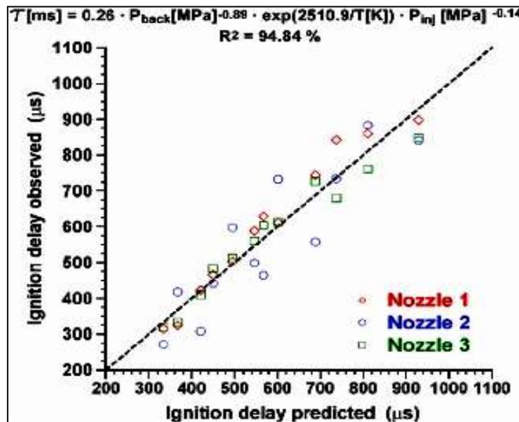
Fig. 8: Observed Vs. Predicted for Ignition Delay Correlation
