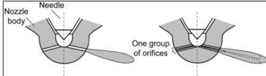
Fig. 1: Concept of a Group-Hole Nozzle (Right) Compared to a Conventional Multi-Hole Nozzle (Left)
