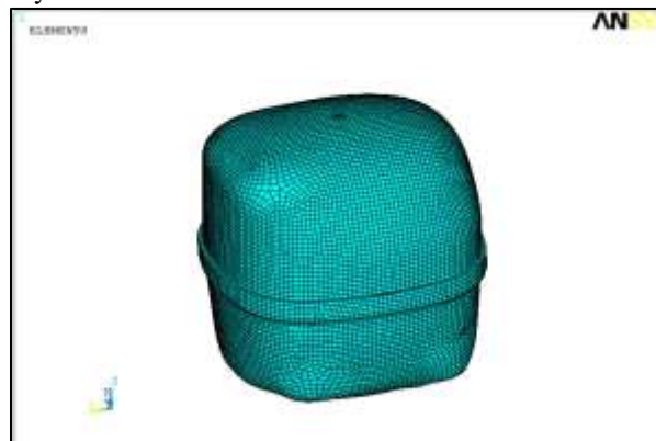
Fig. 2: Shows Finite Element Model of the Shell
