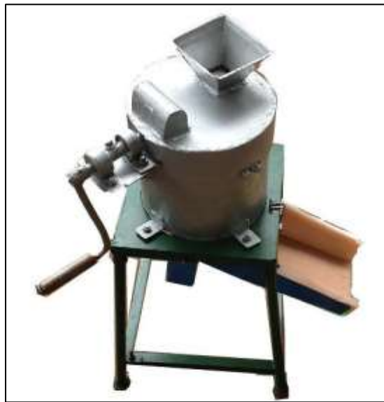
Fig. 2: Roasted groundnut seeds peeling machine
