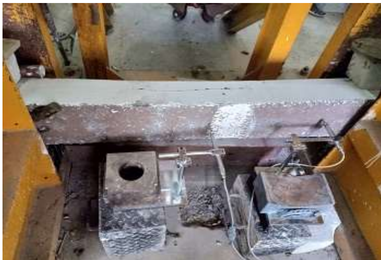
Fig. 2: LVDT Instrumentation Used In Experiment
