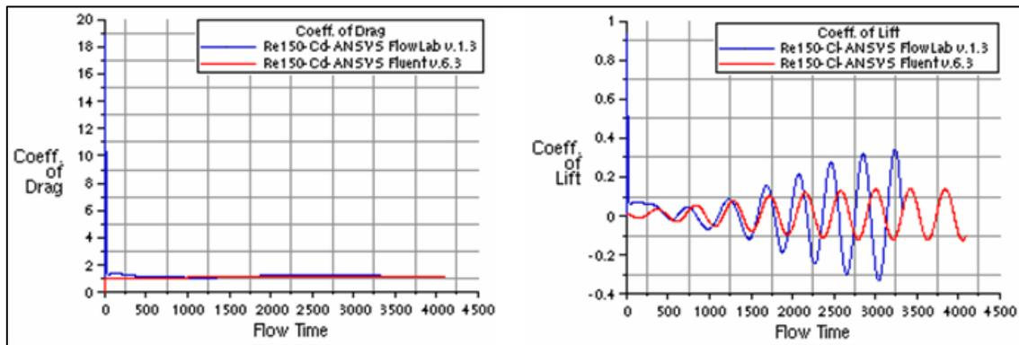
Fig. 6: Validation plots showing coefficient of drag and lift for unsteady state.
