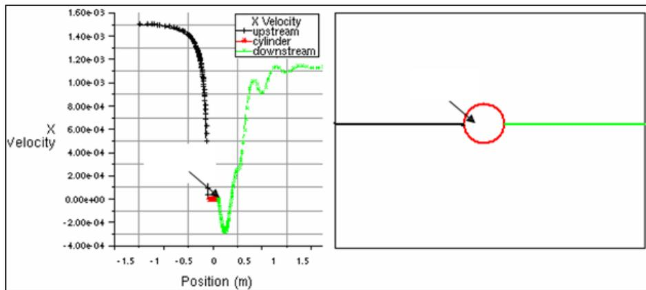
Fig. 4: Center-line Velocity profile in x-direction for a computational domain.
