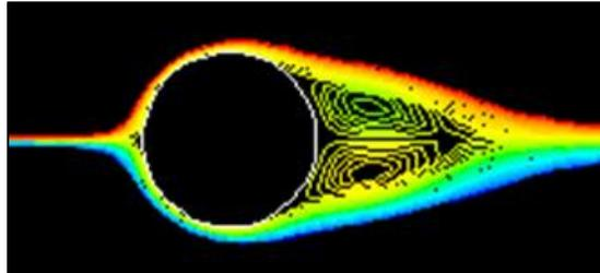
Fig. 3: Contour of Stream function at  $Re < 20$
