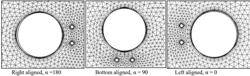
Fig. 2: Alignment of offshore foundation, in a fixed horizontal flow direction.
