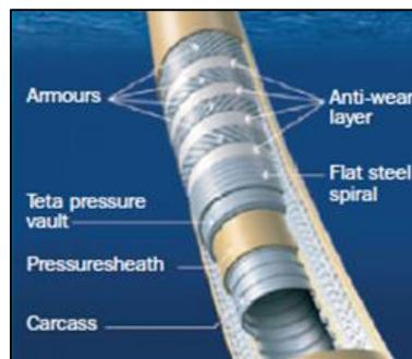
Fig. 1: Flexible riser with carcass profile [1]
