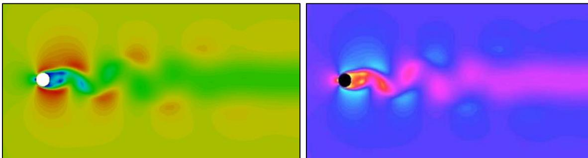
Fig. 5: Plot of velocity magnitude at  $Re = 150$ , Flow time = 4000 seconds, laminar, Positive photo (left), Negative photo (right), ANSYS Fluent Inc.
