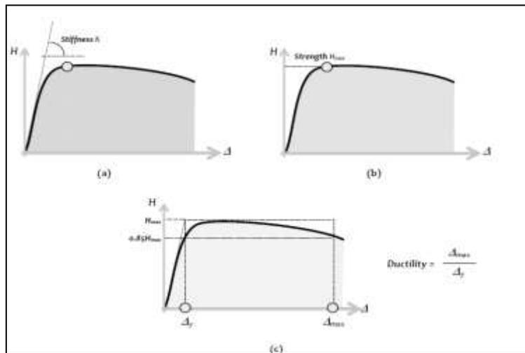
Fig. 3: Structural Characteristics: Overall load deformation curves of a building, indicating (a) lateral stiffness, (b) lateral strength, and (c) ductility towards lateral deformation
