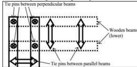
Fig. 5: Overhead view of Kat-Ki-Kuni walls.(Schematic representation of the interconnection between parallel and perpendicular wooden beams)
