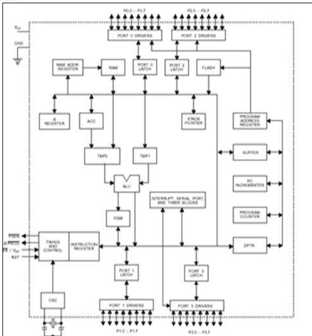
Fig. 4: Architecture of AT89C51 microcontroller
