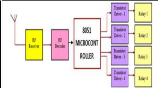
Fig. 2: Control circuit with RF receiver
