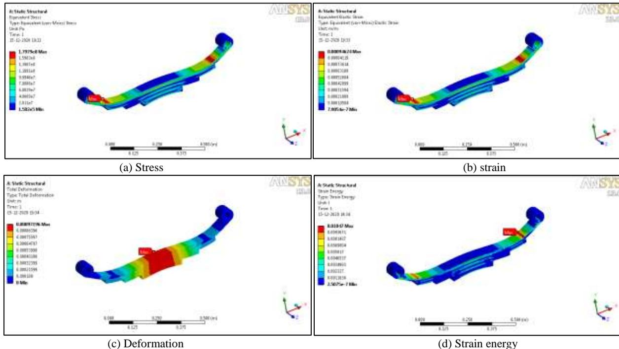
Fig. 5: 50 KN Load-65SI7 Steel Results
