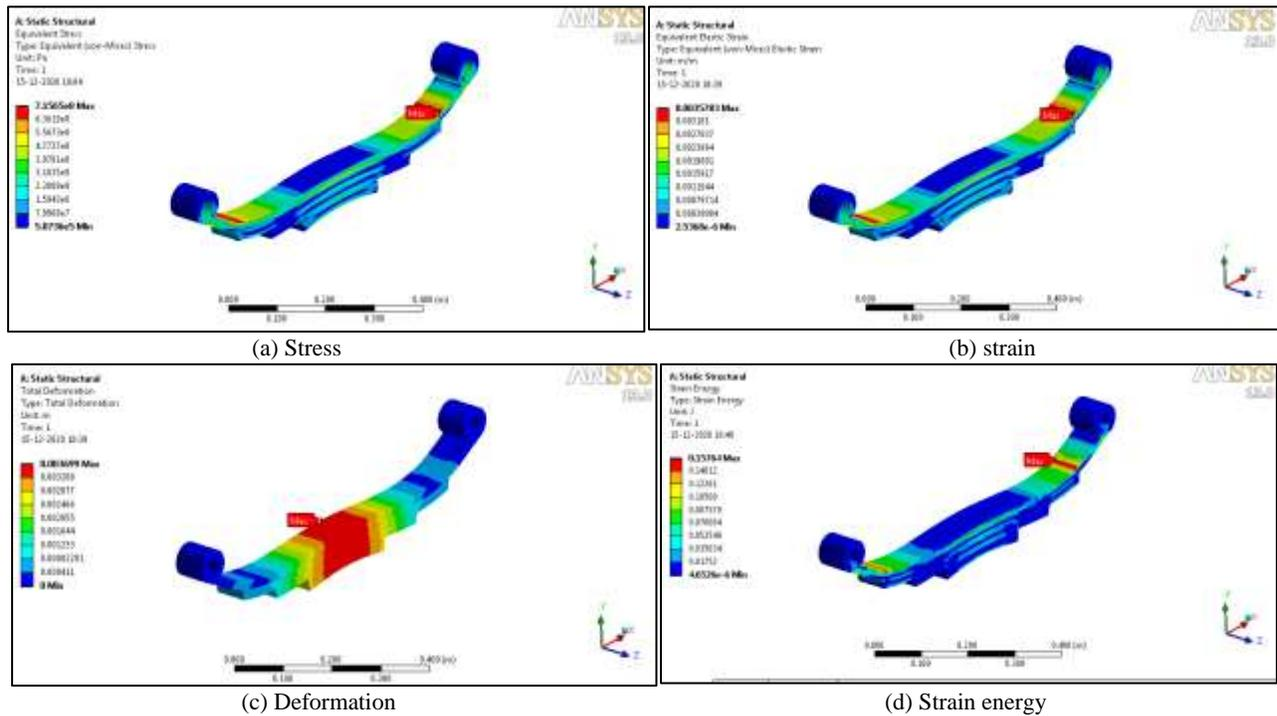
Fig. 6: 200 KN Load Mild Steel Results
