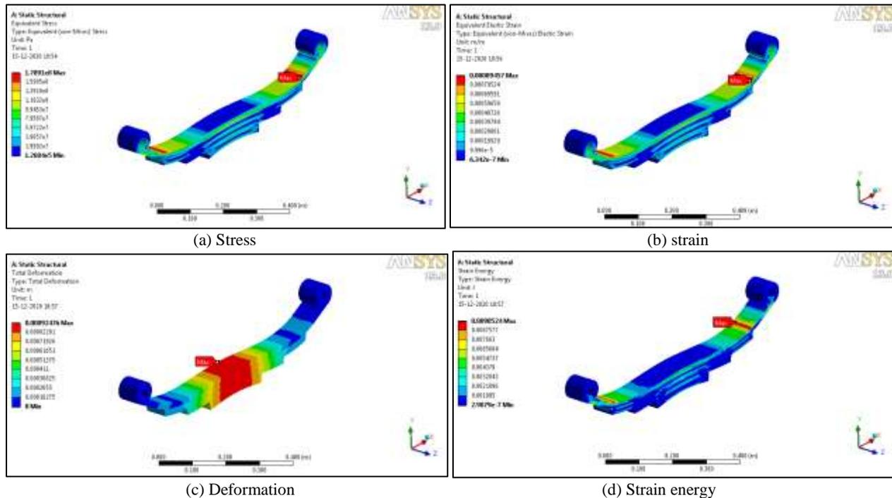
Fig. 8: 50 KN Load Mild Steel Results
