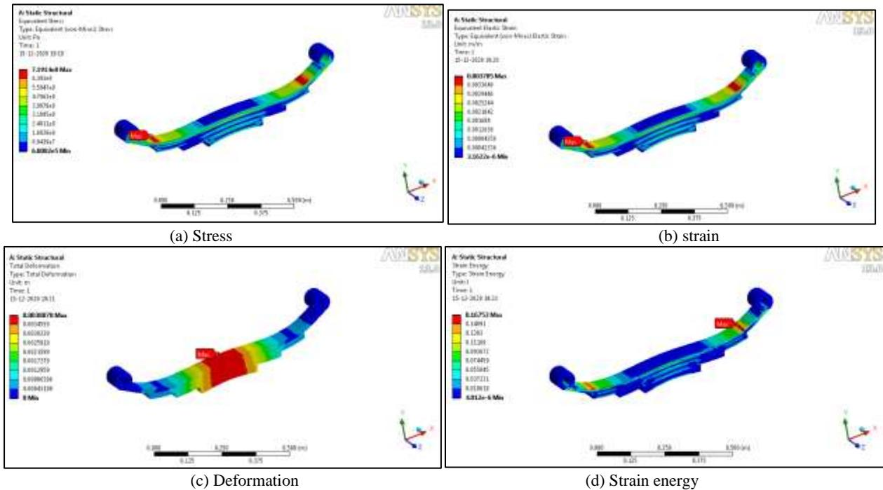
Fig. 3: 200 KN Load-65SI7 Steel Results
