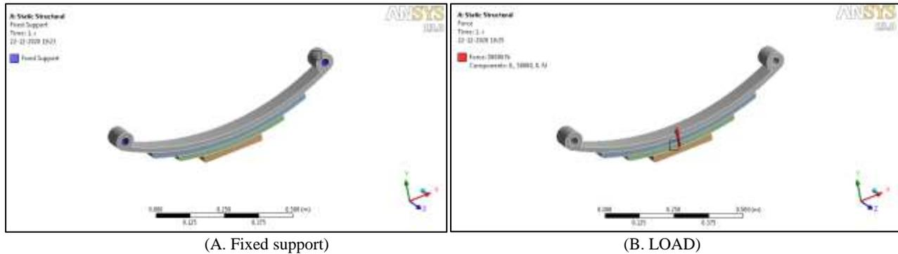
Fig. 2: Loading conditions of specimen
