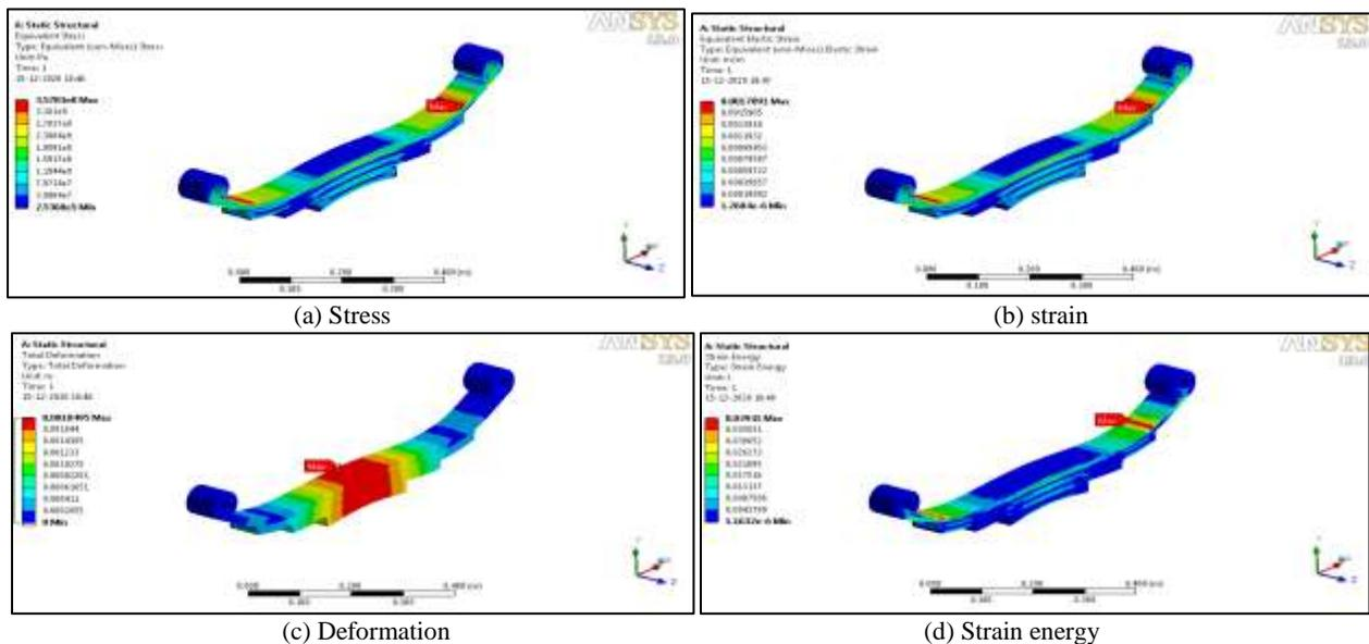
Fig. 7: 100 KN Load Mild Steel Results
