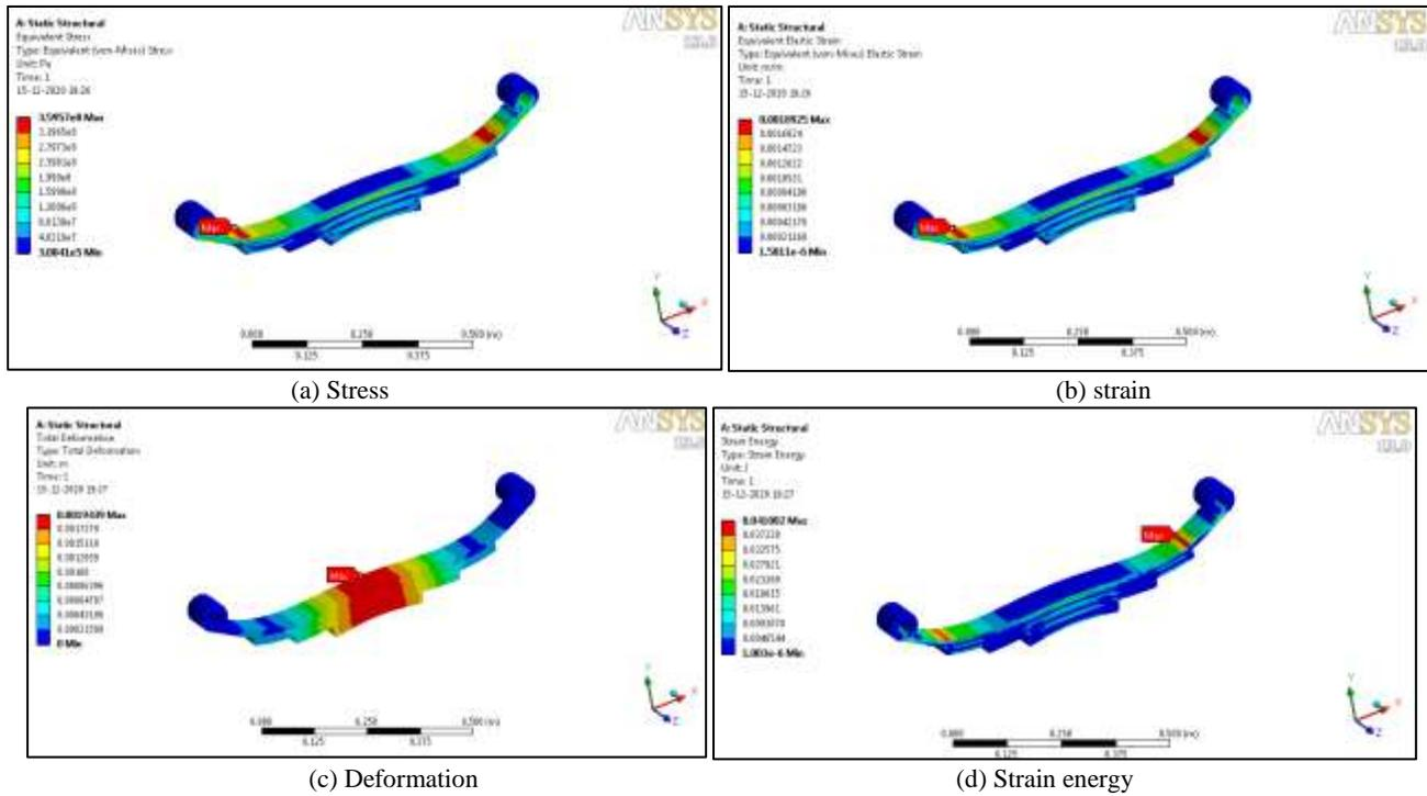
Fig. 4: 100 KN Load-65SI7 Steel Results
