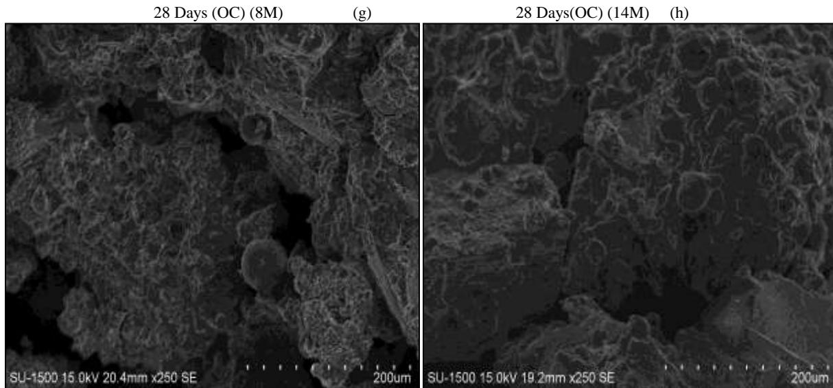
Fig. 14: 28 Days (OC) Comparative SEM Images with NaOH: Na<sub>2</sub>SiO<sub>3</sub> ratio of 1:2.5
