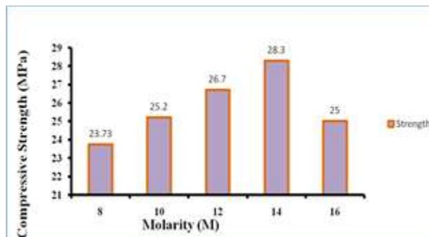
Figure 9 Variation of 28days (Oven cured for 24hours at 800C immediately after casting) Compressive strength
