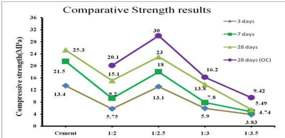
Fig. 10: Variation of Compressive Strength results of cement/ geopolymer mortar of 14M with different NaOH: Na<sub>2</sub>SiO<sub>3</sub> ratios
