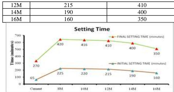
Fig. 2: Setting time of cement paste and different molarities of geopolymer paste with NaOH: Na<sub>2</sub>SiO<sub>3</sub>= 1:2.5
