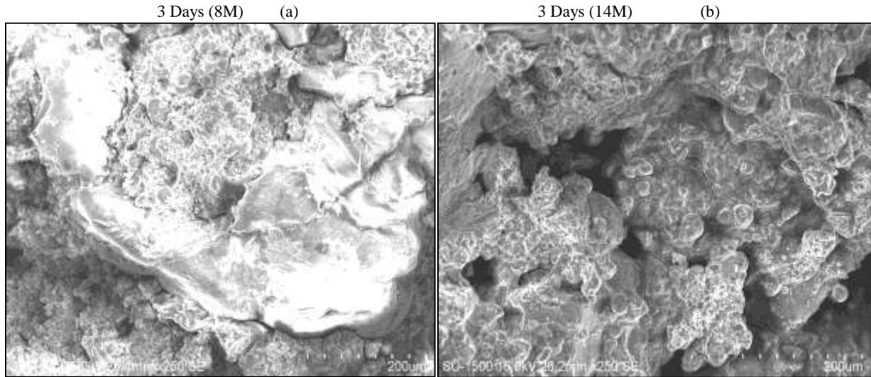
Fig. 11: 3Days Comparative SEM Images with NaOH: Na<sub>2</sub>SiO<sub>3</sub> ratio of 1:2.5
