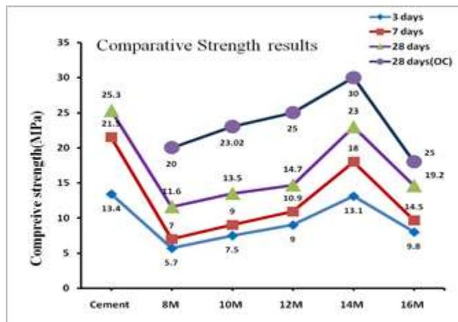
Fig. 5: Comparison of compressive strength of cement/geopolymer mortar different molarities
