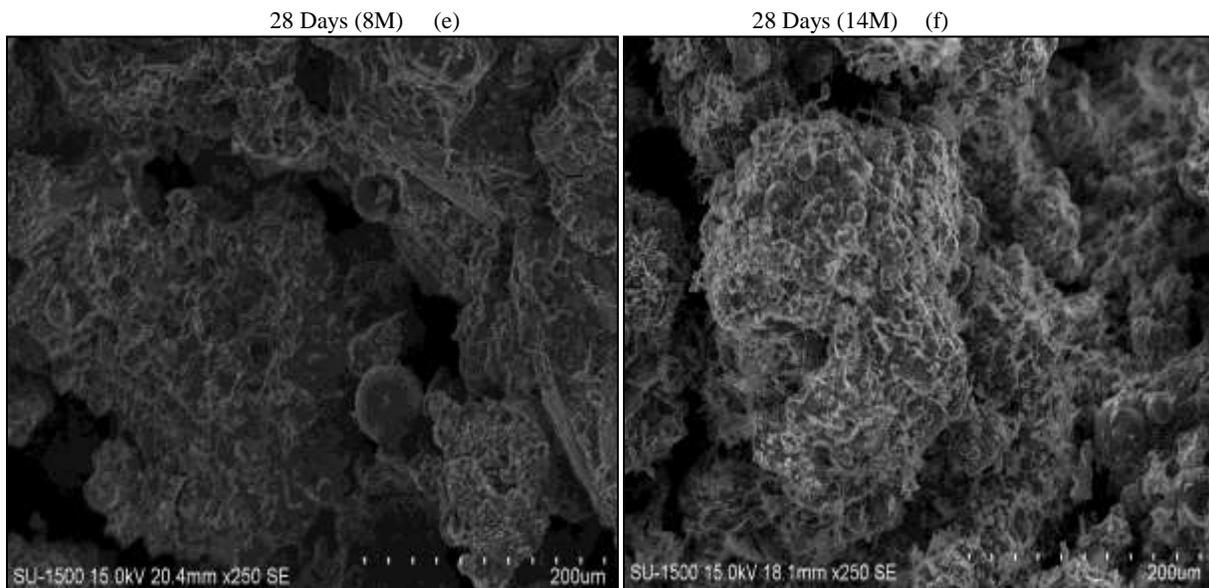
Figure 13: 28 Days Comparative SEM Images with NaOH: Na<sub>2</sub>SiO<sub>3</sub> ratio of 1:2.5
