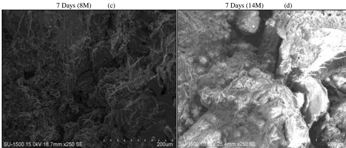
Fig. 12: 7 Days Comparative SEM Images with NaOH: Na<sub>2</sub>SiO<sub>3</sub> ratio of 1:2.5
