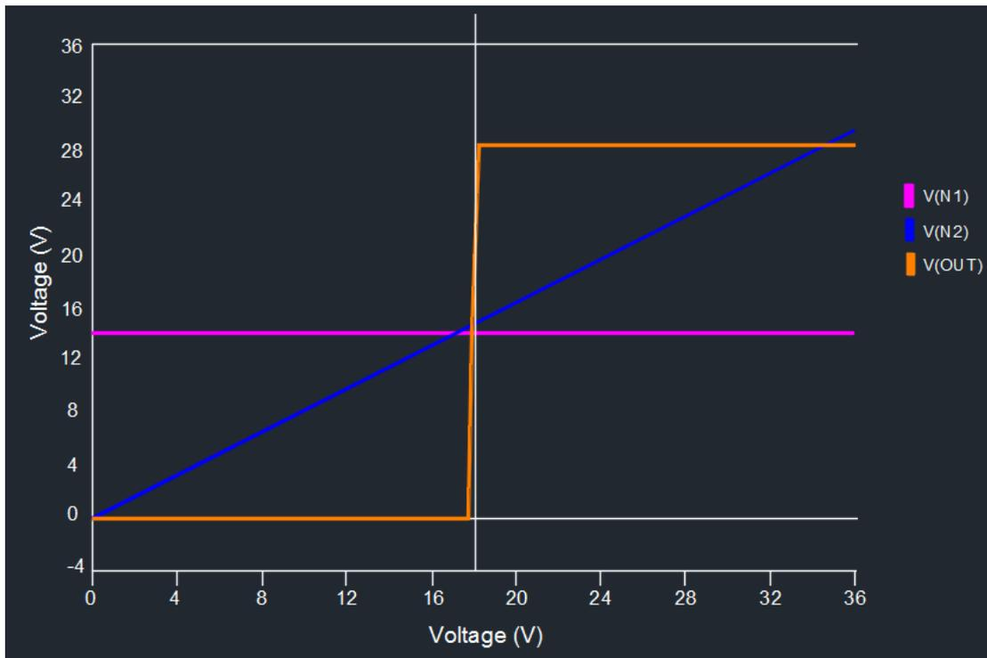
Fig. 3: Dc analysis of CMOS OTA
