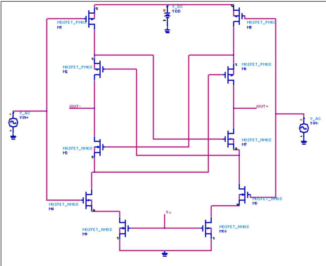
Fig. 5: Feed forward Regulated Cascode OTA
