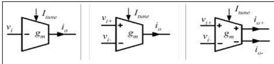
Fig. 1: Three types of OTAs: (a) single-input/output, (b) differential-input single-output, and (c) differential input/output.
