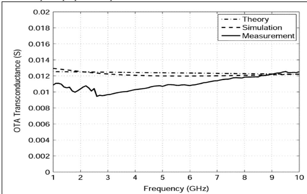
Fig. 7: Proposed OTA's Transconductance
