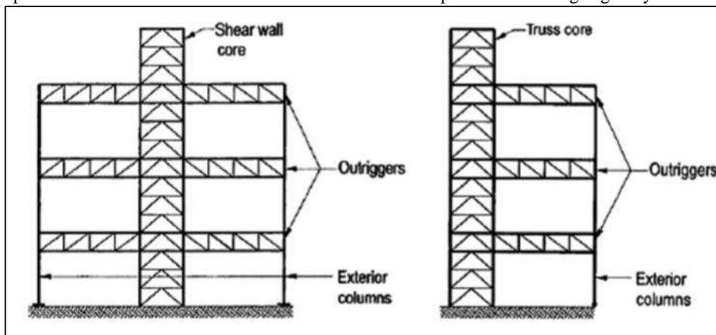
Fig. 02: Outrigger with central core.
