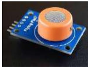
Fig. 2: MQ-03 Alcohol sensor
