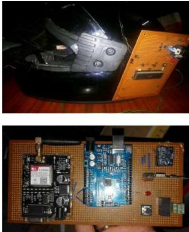
Fig. 6: Circuit in helmet part and bike part
