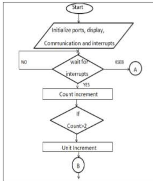
Fig. 3: Flow Chart for Trigger from Energy Meter
