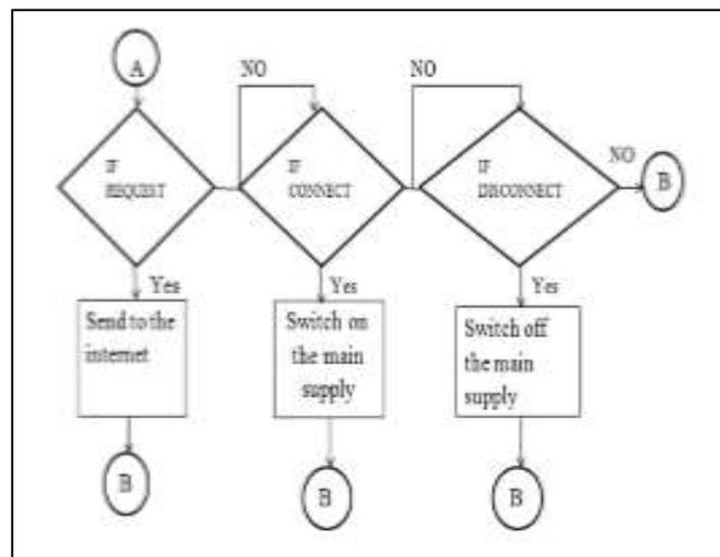
Fig. 4: Flow Chart for Trigger from KSEB
