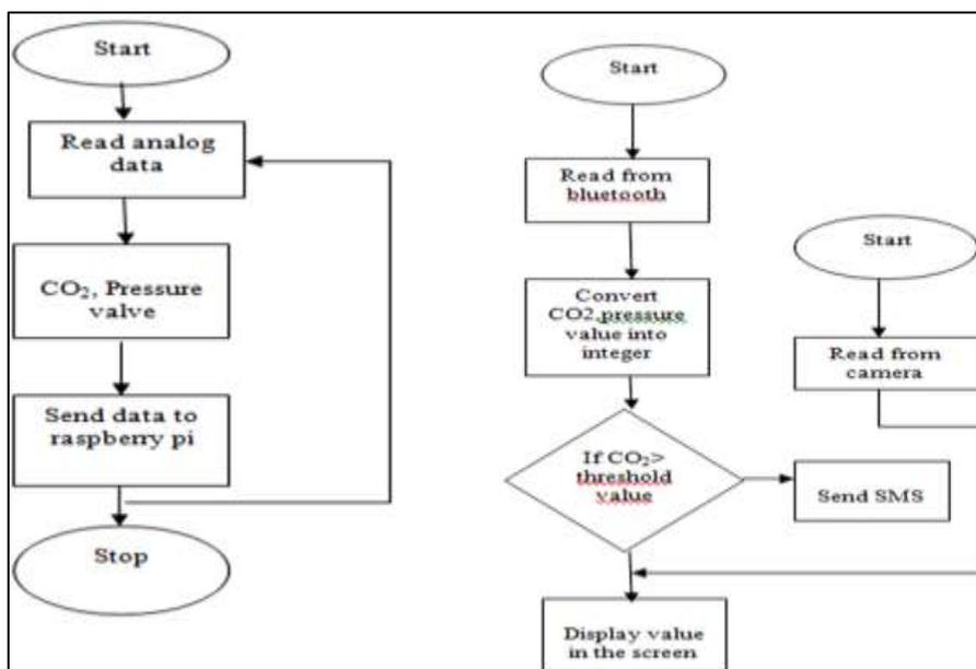
Fig. 3.1: Transmitter Section and Receiver Section
