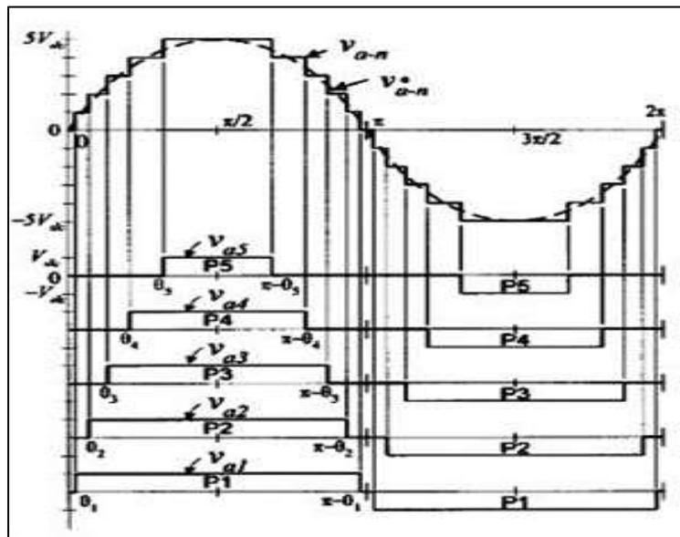
Fig. 2: Output waveform of an eleven level cascaded inverter
