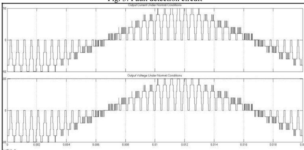
Fig. 4: Output current and voltage under normal conditions
