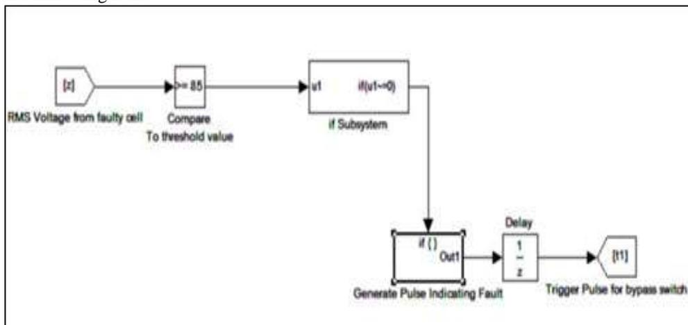
Fig. 3: Fault detection circuit
