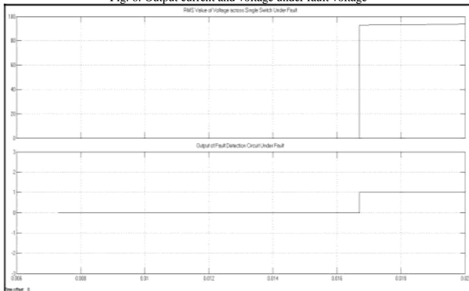
Fig. 7: RMS voltage across a switch and output of fault detector circuit under fault
