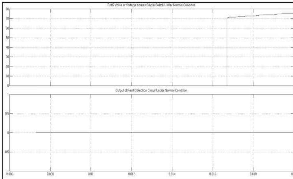
Fig. 5: RMS voltage across a switch and output of fault detector circuit under normal conditions
