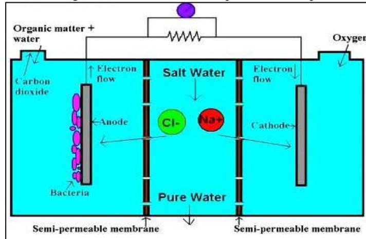
Fig. 2: Circuit digrame of microbial fuel cell
