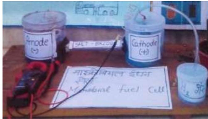
Fig. 1: Microbial Fuel Cell experimental setup
