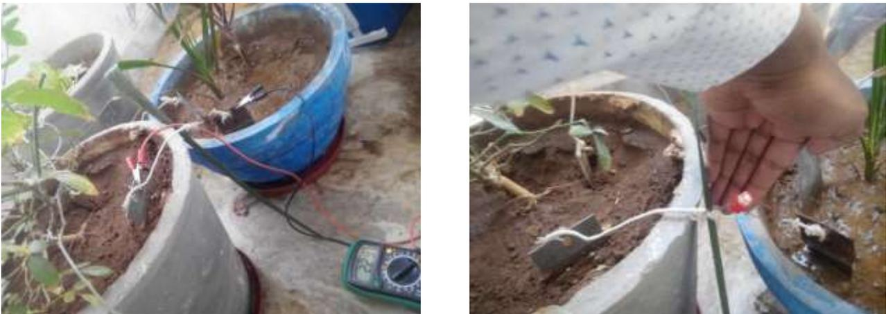
Fig. 3: potential difference generated at 46 hours and the LED consuming power
