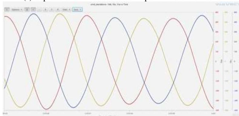
(b) Experimental wave form of three phase output load voltage
