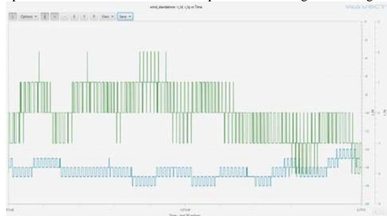
(f) Experimental waveform of d-axis and q-axis stator current of DFIG
