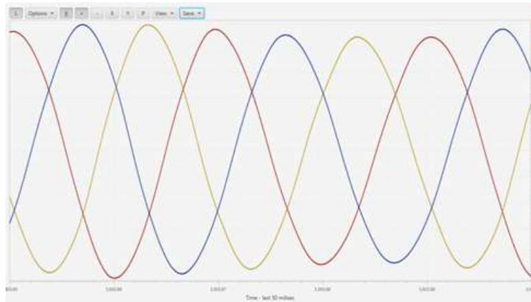
(c) Experimental waveform of three phase output load voltage
