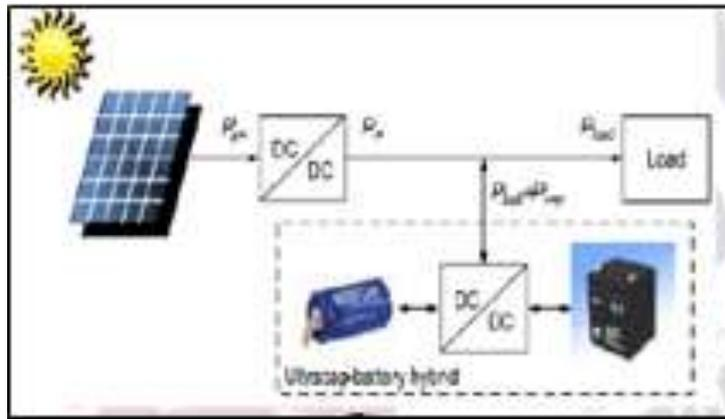
Fig. 4: Solar PV panel using with Battery and super capacitor
