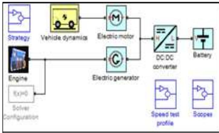
Fig. 2: Series Hybrid Electric Vehicle
