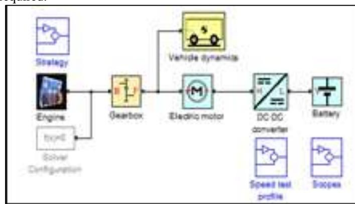
Fig. 3: Parallel hybrid electric vehicle
