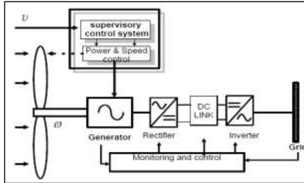
Fig. 2: Variable speed type wind energy conversion
