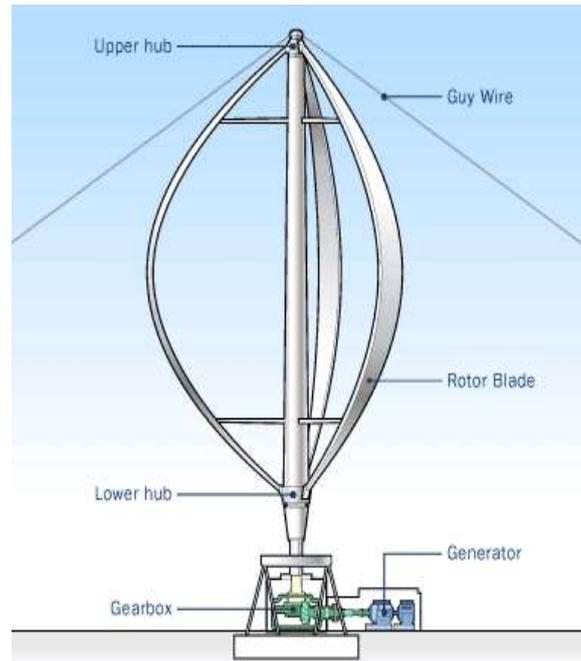
Fig. 6: Components of vertical axis wind turbine (upper hub, guy wire, rotor blade, lower hub, generator, gearbox)
