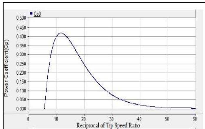
Fig. 3: Performance curve of a wind turbine
