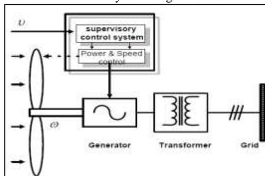
Fig 1: Fixed speed type wind energy conversion system.
