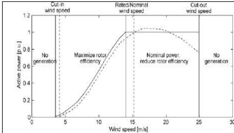
Fig. 4: Typical power curves for a stall controlled (dashed) and pitch controlled (solid) wind turbine
