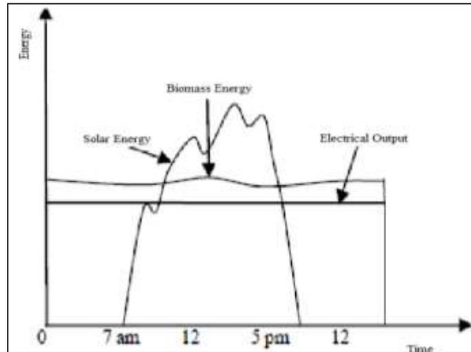
Fig. 1: Characteristics of biomass supported solar power plant
