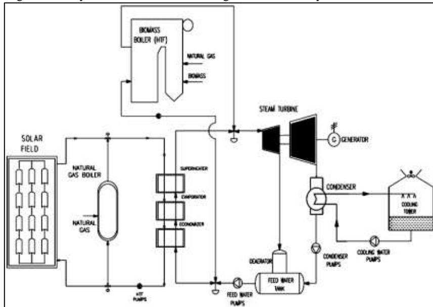
Fig. 4: Solar biomass hybrid configuration with CSP and biomass units set in parallel [1]
