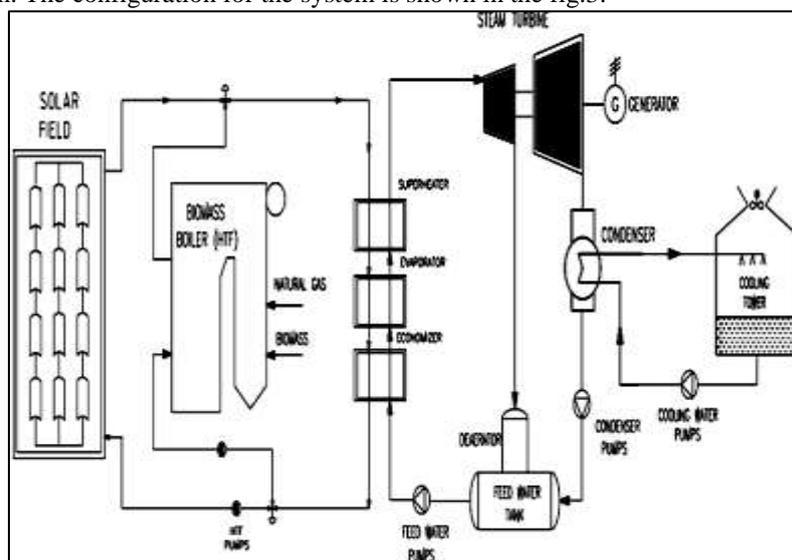
Fig. 3: CSP biomass hybrid configuration in which the natural gas boiler has been substituted by a biomass boiler[1]
