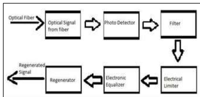
Fig. 1: Block diagram for the electronic equalizer
