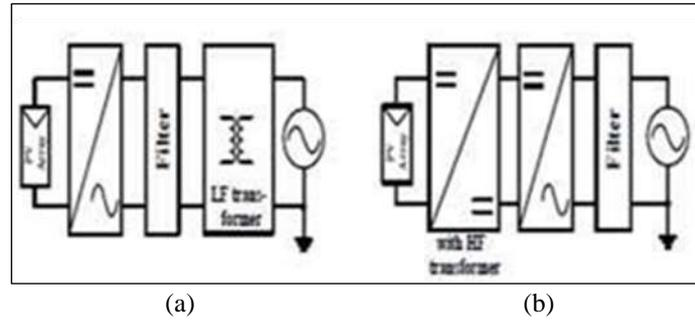
Fig. (2): Grid connected PV system inverter (a)low frequency (LF) transformer (b) high frequency (HF) transformer
