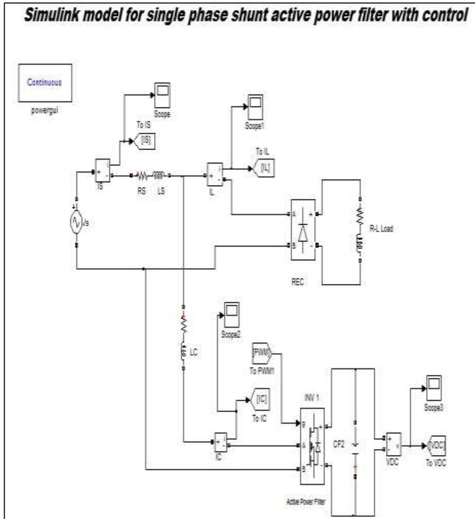
Fig. 4: Simulation circuit of single phase shunt active power filter
