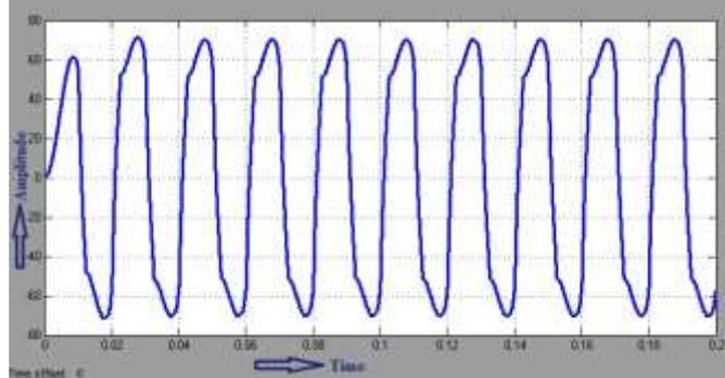
Fig. 6: Load Current of Single Phase Shunt Active Power Filter
