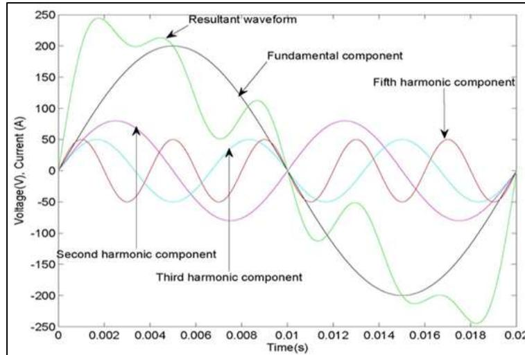
Fig. 2: Components of harmonics in power system
