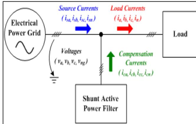
Fig. 1: Basic Building Block of the Active Filter
