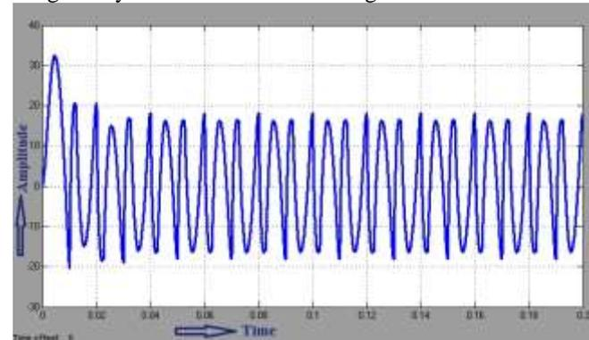
Fig. 8: Compensating Current of Single Phase Shunt Active Power Filter
