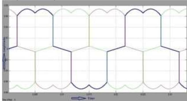
Fig. 11: Load Current for Non Linear Load
