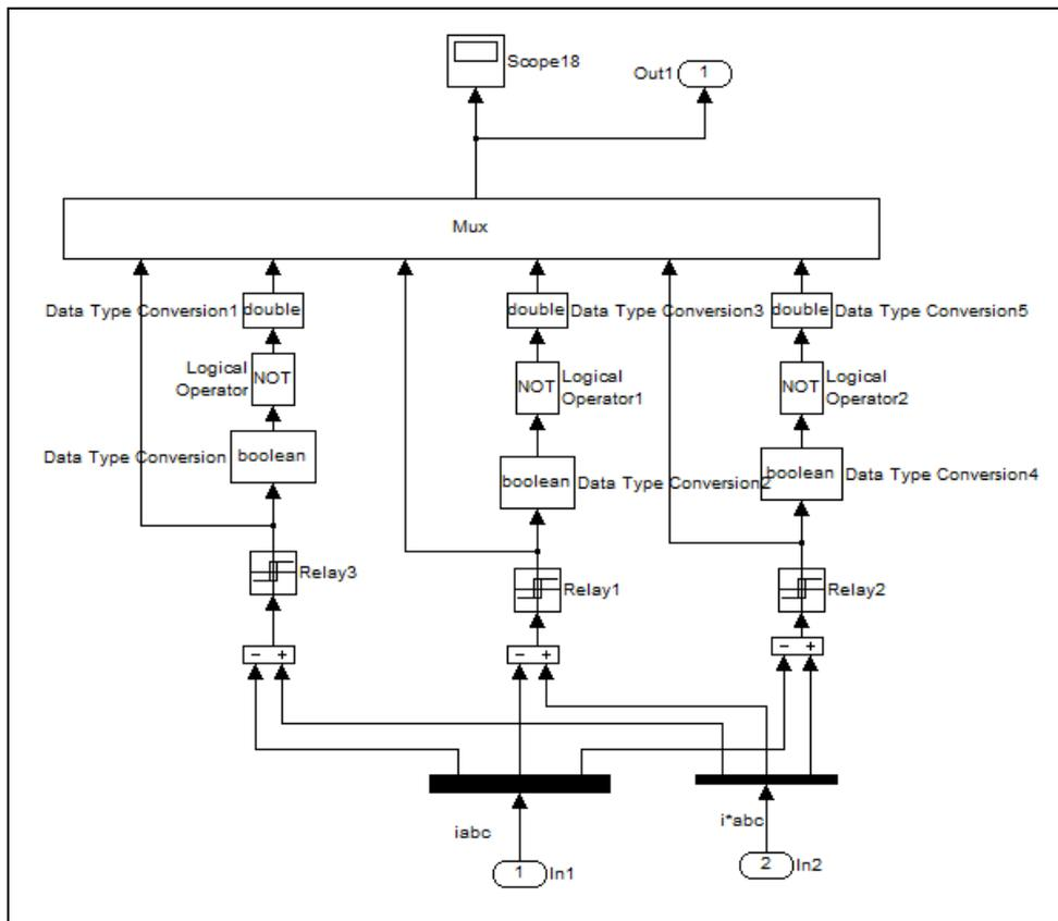
Fig. 3: Circuit of Hysteresis Controller
