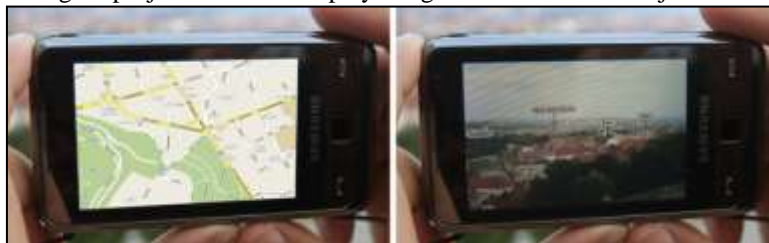
Fig. 2: Contrary to traditional map displays (left), AR 2.0 will augment navigation information on top of the images captured by mobile phones (right). Users will also be able to create and update 3D registered content, creating a location-based social network.
